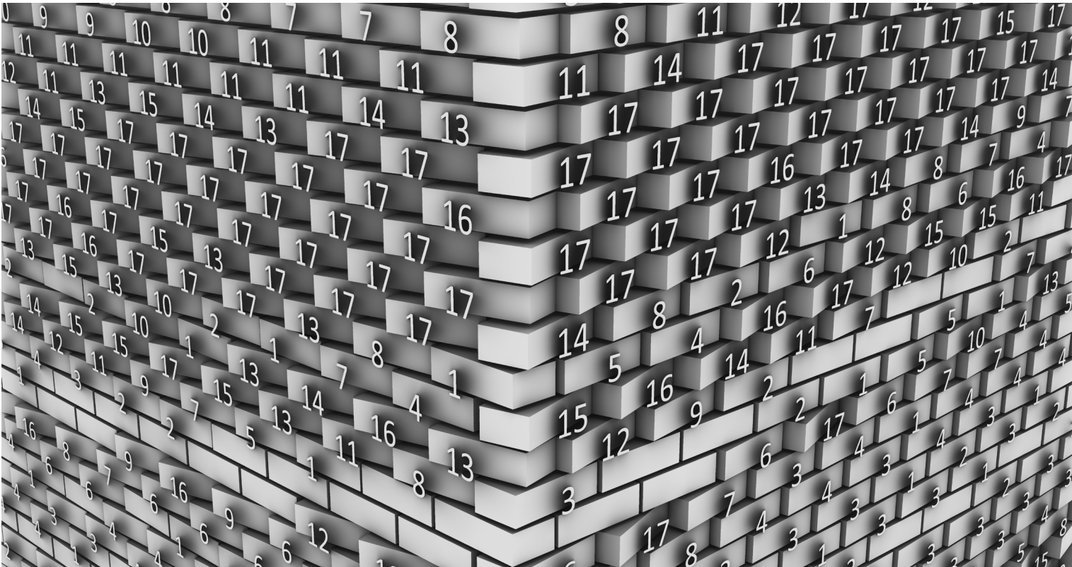
Projected numbering of simplified brick rotations - Bricks only rotate at whole degree numbers for ease of measurement
